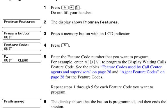
Use the paper labels that come with your telephone to identify the programmed button. To use the Feature Code, press the labeled button.
